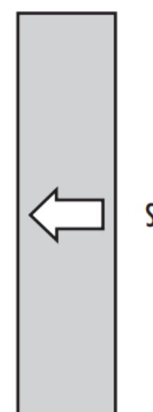
All mounted TECHSPEC® Optical Filters have an arrow on the side of the mount that points to the filter-coated surface for quick reference. Filter oriented such that arrow points to filter coated surface S1.
