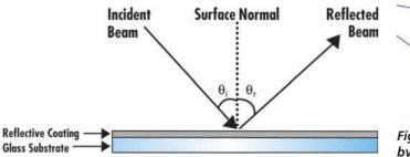
Figure 1: Angle of Incidence ( $\theta_i$ ) = Angle of Reflection ( $\theta_r$ )
