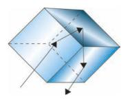
Figure 3: Three mirrors arranged in a right angle "corner" configuration will return a beam back to its source (with some offset) from any incident angle as long as all three mirrors are hit successively
