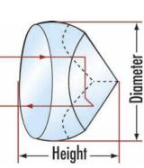
Figure 4: A corner cube retroreflector prism
