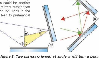
Figure 2: Two mirrors oriented at angle  $\alpha$  will turn a beam by an amount twice that angle. In the special case shown on the right hand side, a 90° orientation will turn the beam 180°
