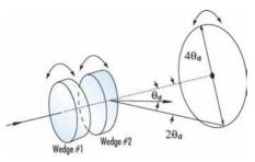
Figure 8: Beam steering in a Risley prism is accomplished by rotating the wedge prisms independently of each other
