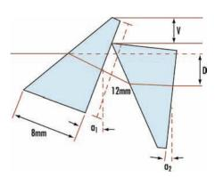
Figure 7: An anamorphic pair uses two tilted wedge prisms to expand a laser beam in one dimension or change its ellipticity
