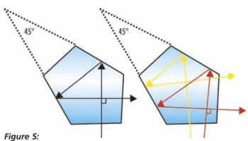
A penta prism has two reflective surfaces oriented at 45°, which produces a 90° beam deviation regardless of the input angle
