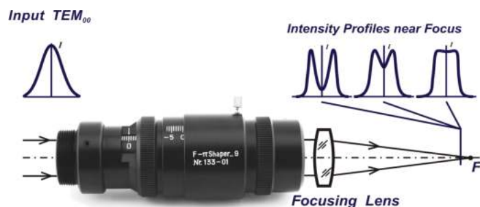
Fig. 2 Principle of the Focal- \pi Shaper operation.
